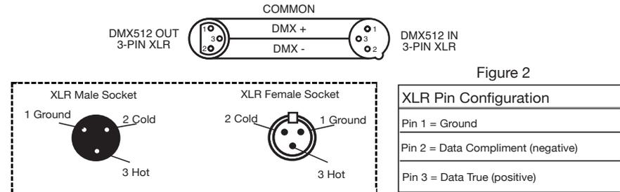
**Special Note: Line Termination.** When longer runs of cable are used, you may need to use a terminator on the last unit to avoid erratic behavior. A terminator is a 90-120 ohm 1/4 watt resistor which is connected between pins 2 and 3 of a male XLR connector (DATA + and DATA -). This unit is inserted in the female XLR connector of the last unit in your daisy chain to terminate the line. Using a cable terminator (ADJ part number Z-DMX/T) will decrease the possibilities of erratic behavior.
