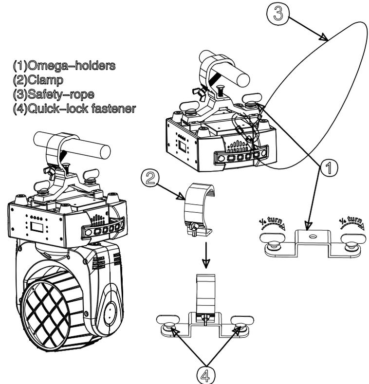
Screw one clamp via a M12 screw and nut onto the Omega holder. Insert the quick-lock fasteners of the Omega holder into the respective holes on the bottom of the Vortex 1200. Tighten the quick-lock fasteners fully clockwise. Pull the safety-cable through the eyehole hook on the bottom of the base and over the trussing system or a safe fixation spot. Insert the end in the carabine and tighten the safety screw.
